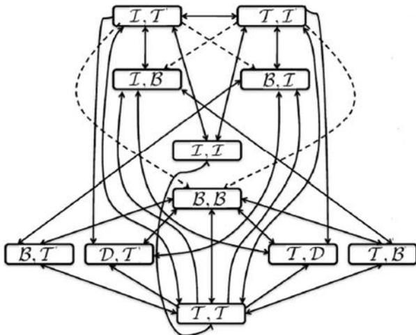
Fig. 4 Markov model of the combined MAC layer behaviour of two nodes [6]
